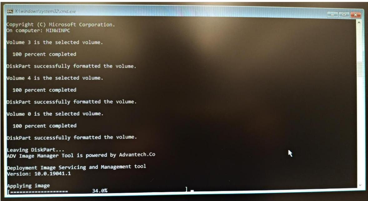
When the recovery is finished, the system will auto restart and boot into Windows. In Windows, open the ADV Image Manager application to check the recovery result.
