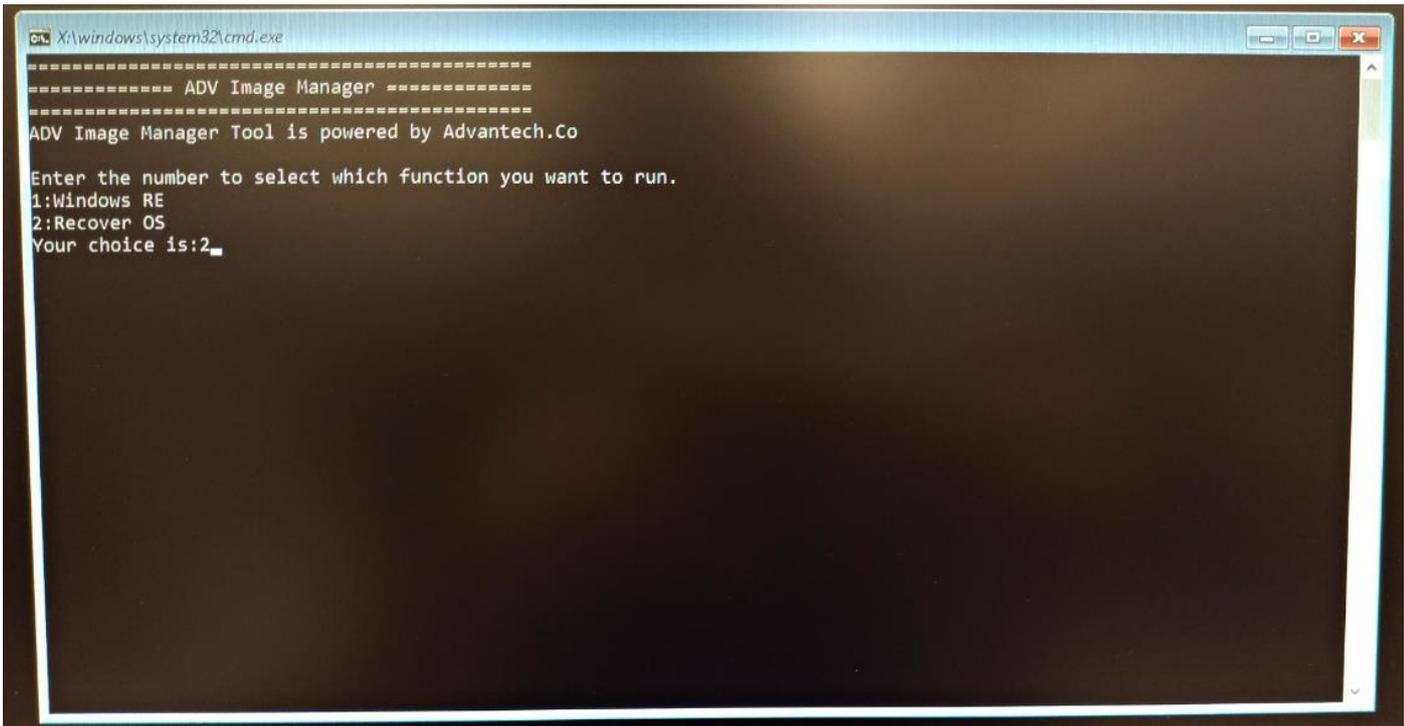
Type "Y" or "y" then press "Enter" to start recovery. After recovery, the system will reboot into Windows.
