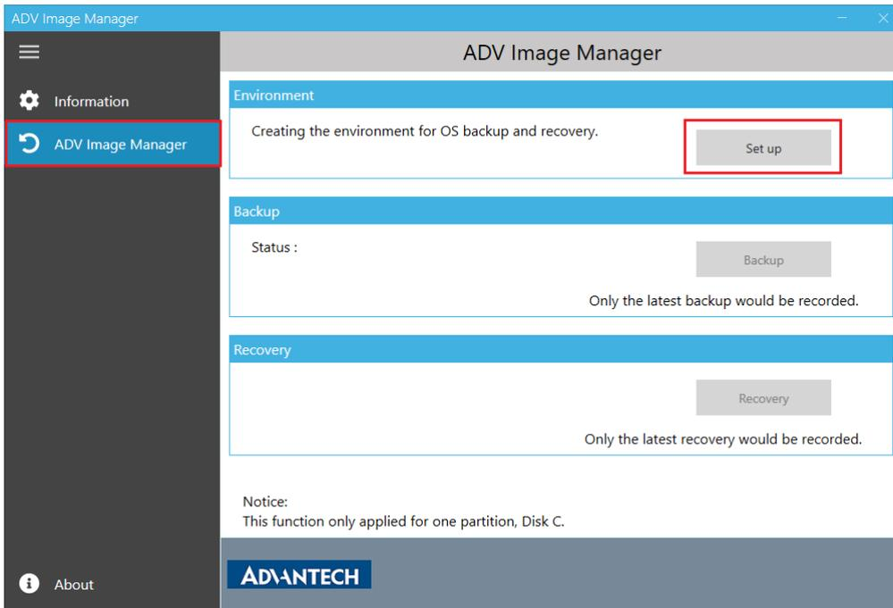
The computer built-in WinRE will be replaced after the ADV Image Manager environment is created. This is an irreversible change even when the ADV Image Manager is uninstalled. Press “OK” to continue creating the environment.
