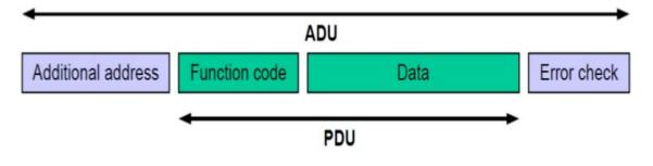
However, the Modbus TCP/IP does not have the Error check part because it already has the checksum protection mechanism.
