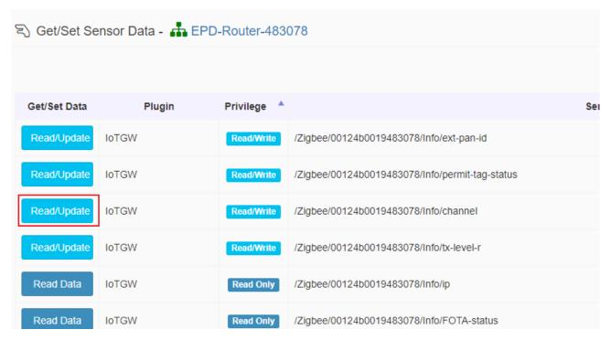
Step 13: You can change the WISE-3240 Channel. Regarding how to select the channel, please reference the other document "EPD Deploy Guide - How to estimate the deployment of ePaper Manager system.pdf"
